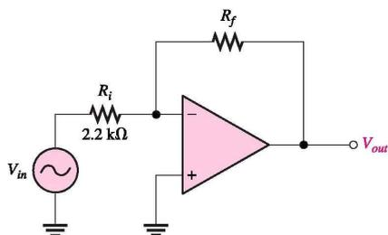
[답]  $|A_{d(NI)}| = \frac{R_f}{R_i} \therefore R_f = 220[k\Omega]$
